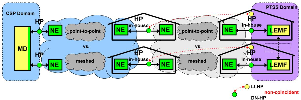
Figure 5 Concatenated delivery network with in-house handover point
