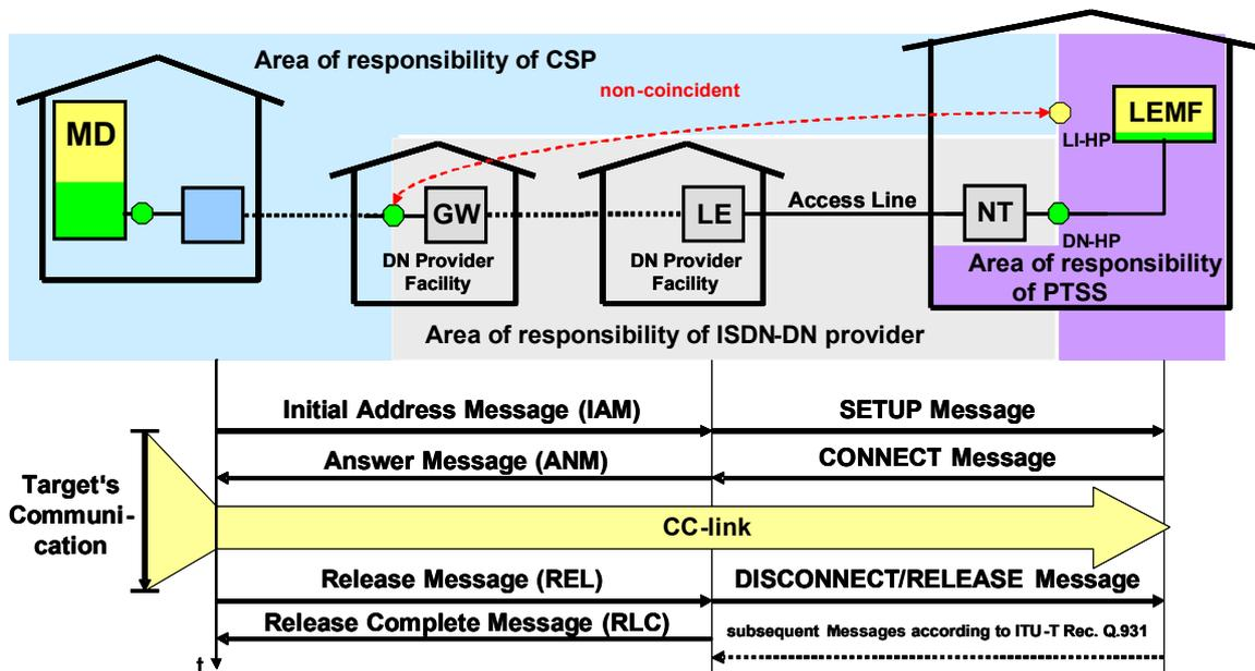
Figure 22 Signalling sequences for the required set-up and release of a CC link
