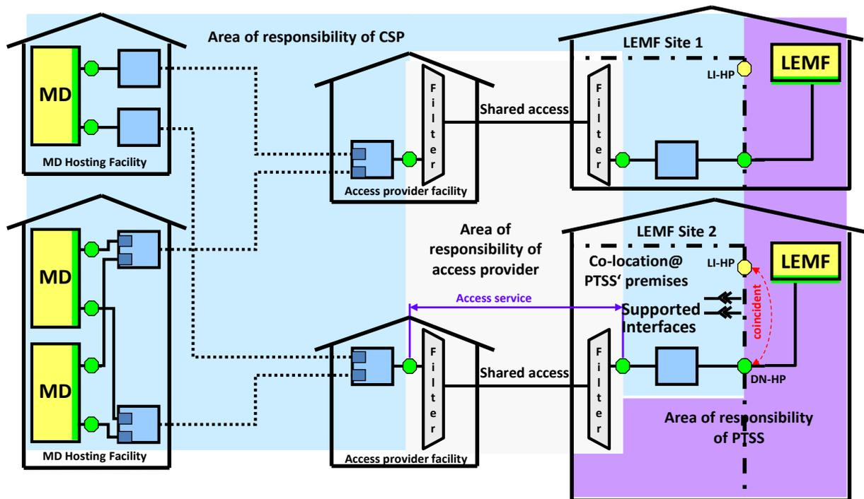
Figure 16 End-to-End view of shared access infrastructure
