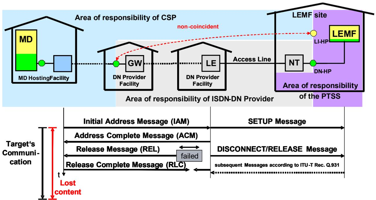
**Figure 24 Signalling sequences for release during set-up of a CC link by the ISDN delivery network**
